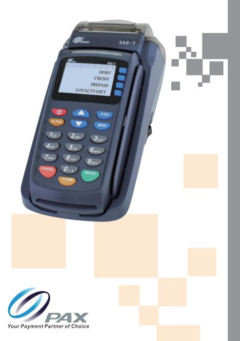
PAX's S60-T is a unique device featuring a compact, ruggedized and yet lightweight POS terminal into a docking station with communications and high-speed thermal printer (or optional sprocket printer).
